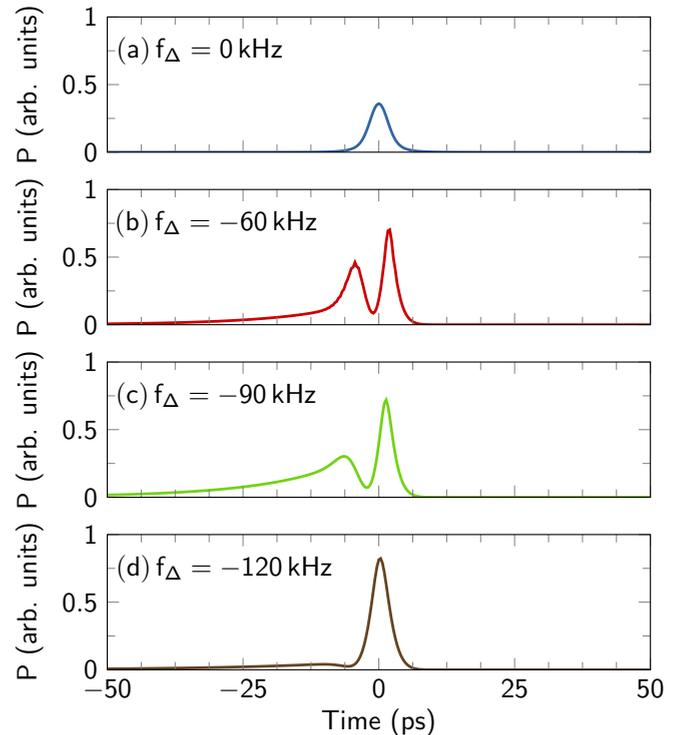
FIG. 5. Numerical simulation showing the variation of the pulse shape power  $P$  for various values of the frequency mismatch  $f_{\Delta}$ . The parameters for the numerical simulations are the same as those in Fig. 4.
