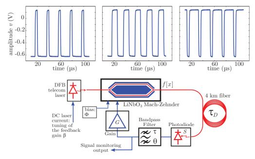
FIG. 1. (Color online) Upper:  $\tau_D$ -periodic square-wave oscillations for three values of the feedback phase  $\phi$  increasing from left to right. The duty cycle is monotonically modified, but the period is unchanged. Lower: Experimental setup performing a bandpass electro-optic Ikeda dynamics.
