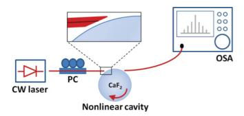
FIG. 1. (Color online) Optical-frequency comb generator with a calcium fluoride cavity and angle-polished fiber couplings. CW, continuous-wave; PC, polarization control; OSA, optical spectrum analyzer. The OSA displays the spectrum of the optical-frequency comb.
