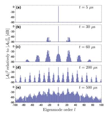
FIG. 11. (Color online) Transient dynamics of the comb when the cavity is pumped with  $|\mathcal{A}_{0s}|^2=1.8\,|\mathcal{A}_0|_{th}^2$ . The parameters are  $\zeta=2\pi\times400$  Hz and  $\sigma=0$ .
