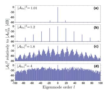
FIG. 10. (Color online) Evolution of the full comb as the pump power in the central mode is increased. The displayed combs correspond to spectrum snapshots at t=2 ms. The parameters are  $\zeta=2\pi\times400$  Hz and  $\sigma=0$ . The  $|\mathcal{A}_{0s}|^2$  is expressed in units of the threshold power  $|\mathcal{A}_0|_{\mathrm{th}}^2$ .
