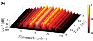
FIG. 12. (Color online) Spectrotemporal behavior of the full comb with  $\zeta=2\pi\times 400$  Hz and  $\sigma=0$ . (a)  $|\mathcal{A}_{0s}|^2=1.2\,|\mathcal{A}_0|_{\text{th}}^2$ , the spectral components converge toward constant values; (b)  $|\mathcal{A}_{0s}|^2=1.8\,|\mathcal{A}_0|_{\text{th}}^2$ , the spectrum is chaotic in the time domain. Note that snapshots at t=2 ms would correspond to Figs. 10(b) and 10(c), respectively.
