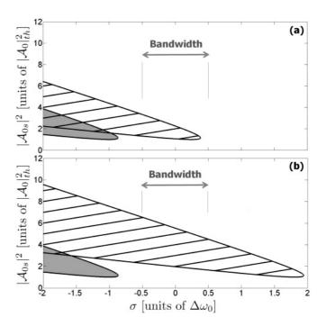
FIG. 7. Stability diagram of various pairs of side modes in the anomalous dispersion regime, with  $\zeta = 2\pi \times 400$  Hz. Hatched and shaded areas have the same meaning as in Fig. 6, and this figure can be interpreted as a follow-up of Fig. 6(b) when the side mode order increases: (a)  $l = \pm 20$ ; (b)  $l = \pm 30$ .
