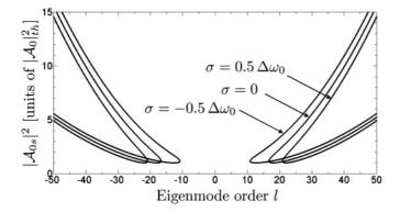
FIG. 9. Various stability diagrams for comb generation as a function of eigenmode order l and power  $|\mathcal{A}_{0s}|^2$  in the central mode, as the laser detuning  $\sigma$  is varied. The dispersion parameter is still set to  $\zeta = 2\pi \times 400$  Hz, and the curve corresponding to  $\sigma = 0$  is exactly the same as the one in Fig. 8. The hatchings have been omitted in this figure in order to improve its clarity.
