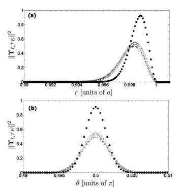
FIG. 3. Radial and polar profiles of the modes (arbitrary units) for  $\ell_0=143\,50$  (plusses), for  $\ell_0+10\,00$  (open circles), and for  $\ell_0+10\,000$  (solid circles). (a) Radial profiles for  $\theta=0$  and  $\phi=0$ . (b) Polar profiles for  $\phi=0$  at intensity maxima. All other parameters are those of Fig. 2.
