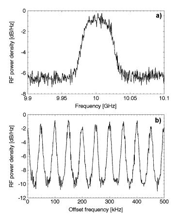
Fig. 4. Experimental power density spectra of the microwave noise below threshold. The spectrum has been scaled to its maximum (reference at  $\sim 0$  dB). (a) Spectrum in a 200 MHz window, showing how the noisy power density is profiled by the RF filter. (b) Zoom-in with near the 10 GHz central frequency in a 500 kHz window, showing the noisy ring-cavity peaks.
