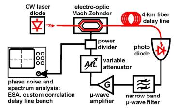
Fig. 1. Experimental setup.
