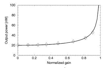
Fig. 2. Variation of the RF noise output power  $\bar{P}_{\gamma}$  as a function of the normalized gain, under threshold. The solid line is the theoretical prediction of (15) with  $D_a = 9.8 \times 10^{-16} \text{ rad}^2/\text{Hz}$ , and the symbols represent the experimentally measured data. The gain was varied through attenuation in the electric branch of the loop.
