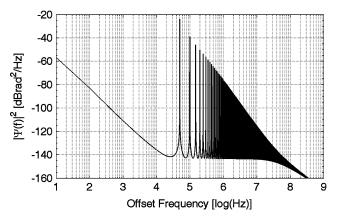
Fig. 5. Theoretical phase noise spectrum above threshold in a 500 MHz window, with  $D_a = 9.8 \times 10^{-16} \text{ rad}^2/\text{Hz}$ ,  $D_m = 5 \times 10^{-11} \text{ rad}^2/\text{Hz}$ ,  $\Omega_H = 100 \text{ kHz}$  and  $\Omega_L = 1 \text{ Hz}$ . The dimensionless amplitude of the microwave oscillation is  $|\mathcal{A}_0| = 0.41$ , corresponding to a power of 10.5 dBm.
